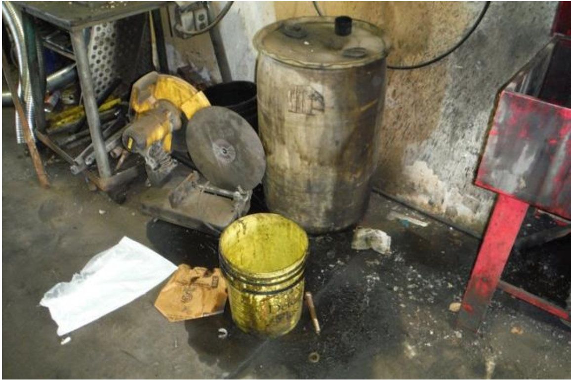
Miscellaneous chemicals stored on shop floor with heavy staining
